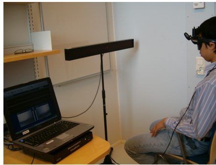
Figure 3 A subject was following the target with his gaze on the bar in front of him. The small red LED was the target light, which jumped abruptly from one place to another along the bar (see online version for colours)
