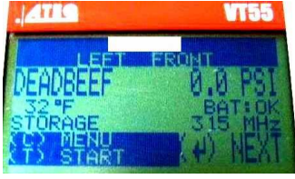
Figure 12: The TPMS trigger tool displays the spoofed packet with the sensor ID “DEADBEEF”. We crossed out the brand of TP sensors to avoid legal issues.
