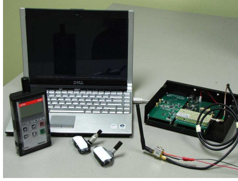
Figure 2: Equipment used for packet sniffing. At the bottom, from left to right are the ATEQ VT55 TPMS trigger tool, two tire pressure sensors (TPS-A and TPS-B), and a low noise amplifier (LNA). At the top is one laptop connected with a USRP with a TVRX daughterboard attached.
